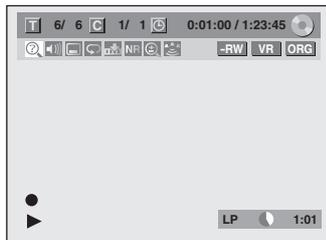
If you play back the fast forward playback and the playback reaches the scene recorded 1 minute before, the forwarding playback will automatically return to the normal playback.
