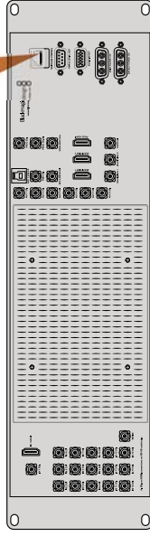
ATEM 1 M/E and 2 M/E Production Switchers have an audio in/out port which connects to an analog audio breakout cable.
