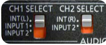
Two switches behind LCD panel
